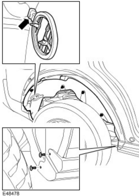
7. Remove the fuel filler door. For additional information, refer to [Fuel Filler Door Assembly \(19.55.04\)](#) (Section 501-03)
