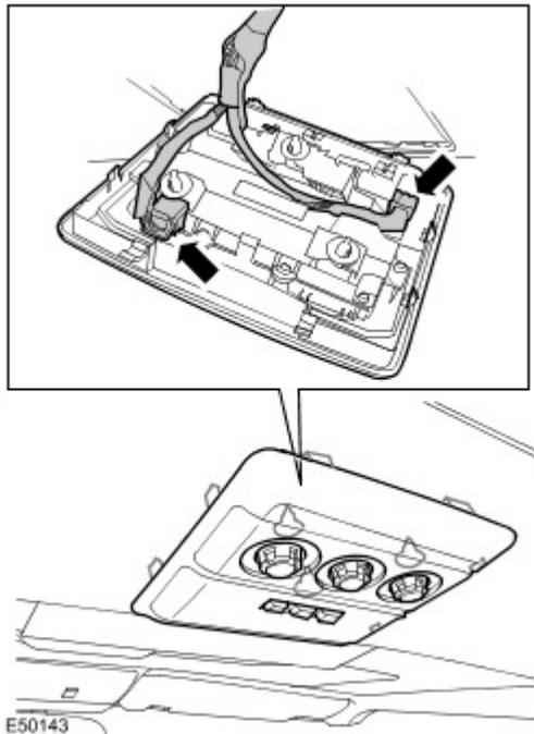
2. Remove the roof opening panel module.
