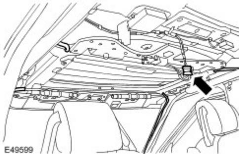
4. With assistance, remove the roof opening panel assembly.
