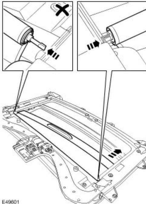
6. Remove the roof opening panel motor.
