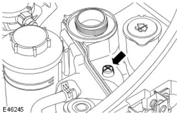
19. Loosen the coolant expansion tank bleed screw.
