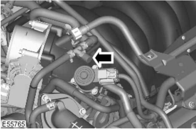
18. Loosen the coolant hose bleed screw.
