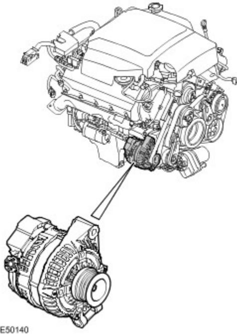
The generator is located at the front RH side of the engine, on the cylinder block. The generator has an output of 85/150 Amps and is manufactured by Denso. A six-ribbed polyvee belt drives the generator pulley, which in turn is driven from the engine crankshaft pulley.
