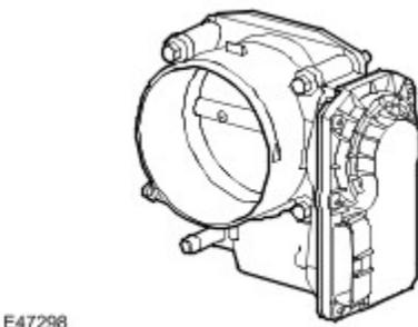
The V8 EMS incorporates an electric throttle control system. The electronic throttle body is located on the air intake
