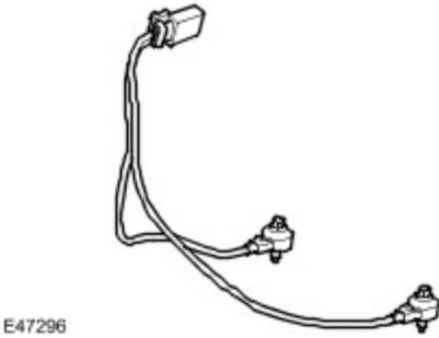
The V8 EMS has two knock sensors located in the V of the engine, one per cylinder bank. The sensors are connected to the ECM via a twisted pair.
