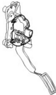
The APP sensors are located on the accelerator pedal assembly.
