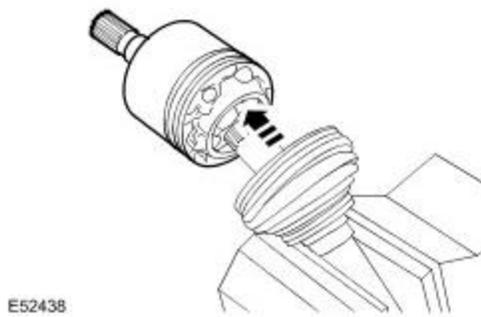
7. Using a drift against the inner part of the CV joint, remove the CV joint from the halfshaft.
