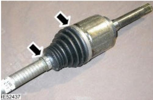
6. Slide the CV joint boot along the halfshaft to gain access to the joint.
