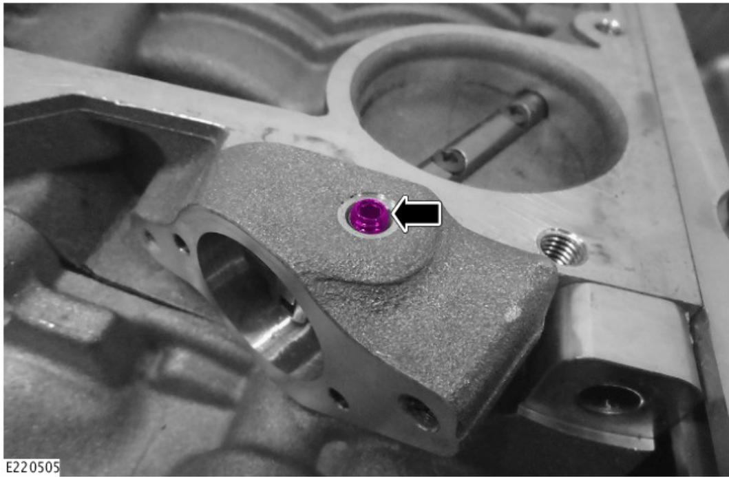
Remove the bypass valve set screw.
