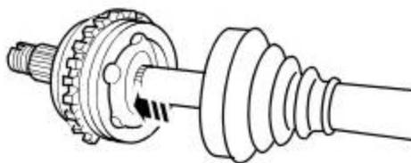
8. Remove the outer CV joint boot.
