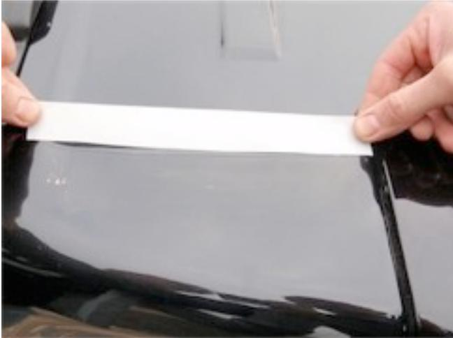
10. Remove the backing from the double sided tape underneath the top step of the ladder.
