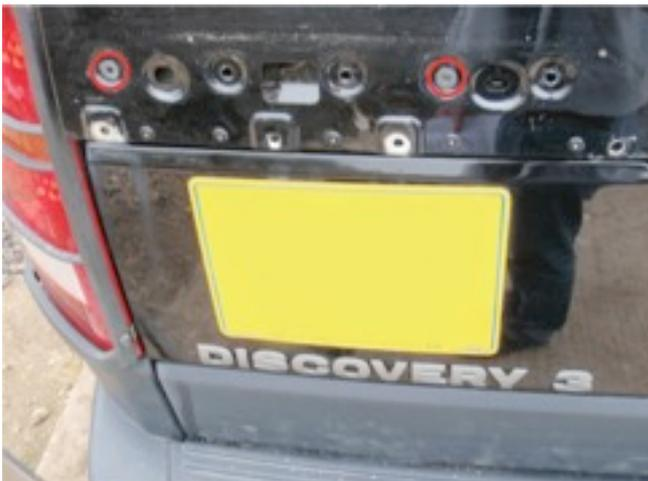
8. Clean off the surfaces ready for mounting the ladder.
