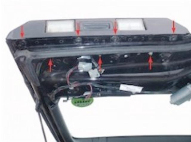
6. Remove the two plastic clips from the panel. Do NOT shut the boot once the handle has been removed.
