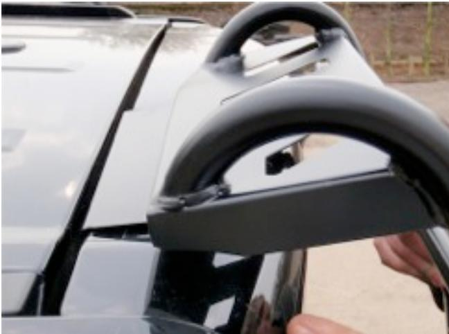
12. Fasten into place using the two hex head bolts each with a washer. Before fully tightening the two bolts check to make sure the ladder is aligned with the lower holes.
