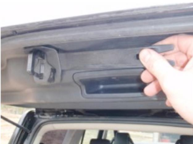
3. Remove the interior plastic panel that runs along the rear door.
