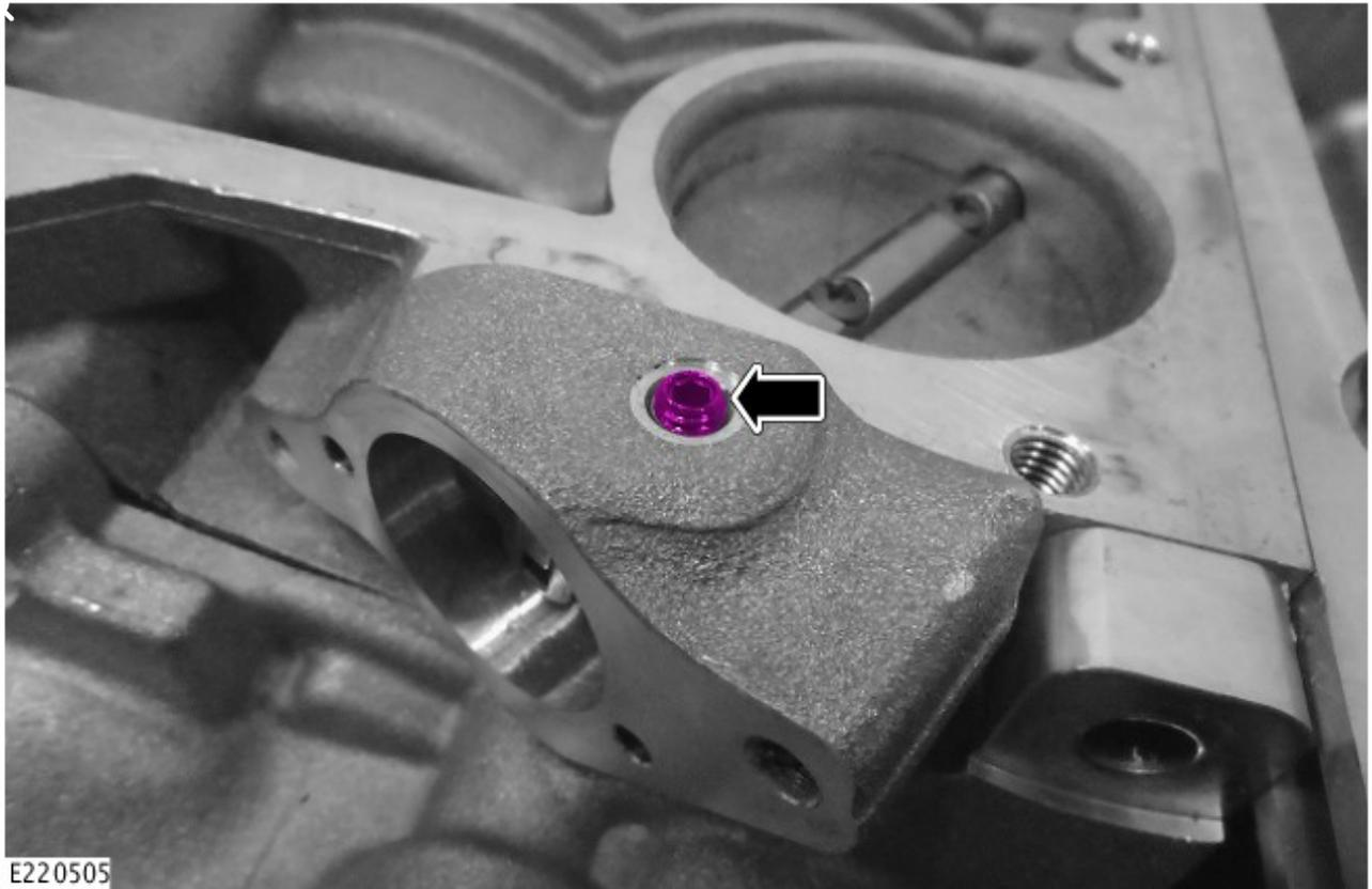
Remove the bypass valve set screw.
